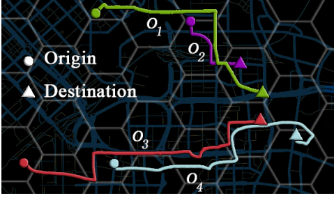
Fig. 1: Example of shareable orders, where different orders traverse the same cell in the same time slot.
